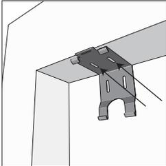
Remove the brackets from the headrail assembly. Align each bracket with your location marks and while holding the bracket in place, mark the mounting screw locations in the top of the bracket with a pencil. Pre-drill marked locations using a 1/8 in. drill bit. Attach the brackets securely using the supplied mounting screws and a Phillips screwdriver.
