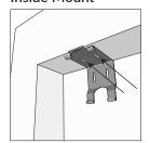
Remove the brackets from the headrail assembly. Align each bracket with your location marks and while holding the bracket in place, mark the mounting screw locations in the top of the bracket with a pencil. Pre-drill marked locations using a 1/8 in. drill bit. Attach the brackets securely using the supplied mounting screws and a Phillips screwdriver.
